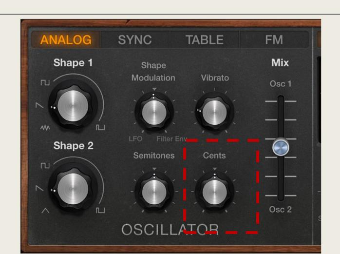
Mix slider: Crossfade (set the level relationships) between the oscillators (Shape 1 and 2).
