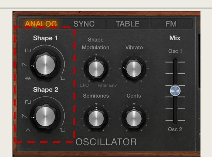
Shape Modulation knob: Choose a waveform shape modulation source, and set the modulation intensity. The centered (off) position disables all waveform shape modulation with the LFO or filter envelope.
